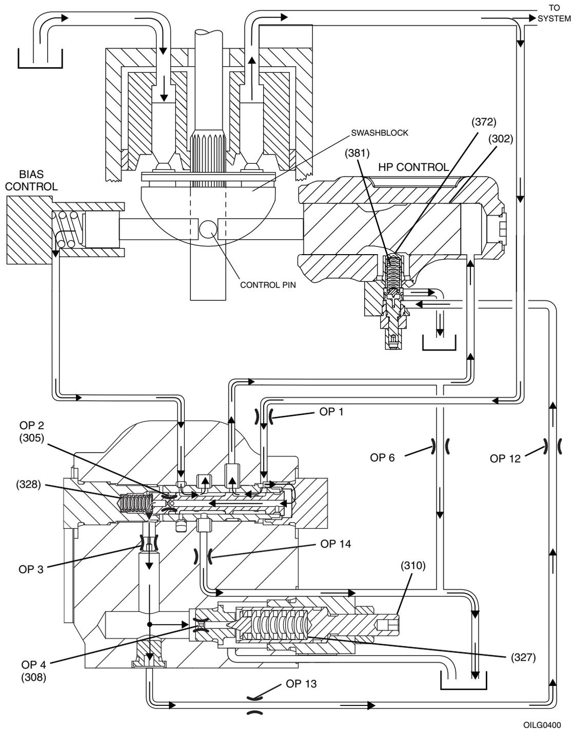
**Figure 6. Compensating Pressure (Unloading) - Horsepower Limiter Active**
