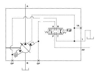
Be sure system and pumps are protected against over loads with a high pressure relief valve.
